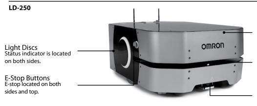
Hardened Construction Metal chassis and skins for increased duty and durability.
